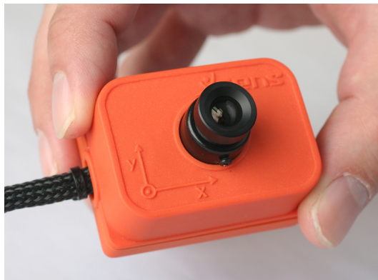
Figure 1: The sensor unit, consisting of an IMU and a camera.
