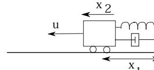
A mechanical system with nonlinear spring and position-dependant damping.
