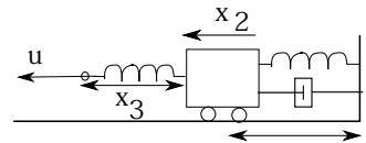
A mechanical system with two nonlinear springs and position-dependant damping.
