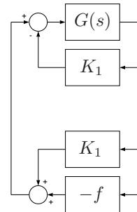
The system  $G$  with feedback  $f$  is equivalent to  $G(I + K_1 G)$  having the feedback  $f - K_1 y$ .
