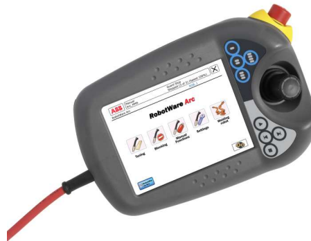
Figure 2.7 An example of a teach pendant: The ABB IRC5 FlexPendant (ABB, 2004).
