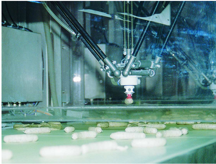
Figure 2.2 Picking sausages with the ABB Flexpicker (ABB, 2004).
